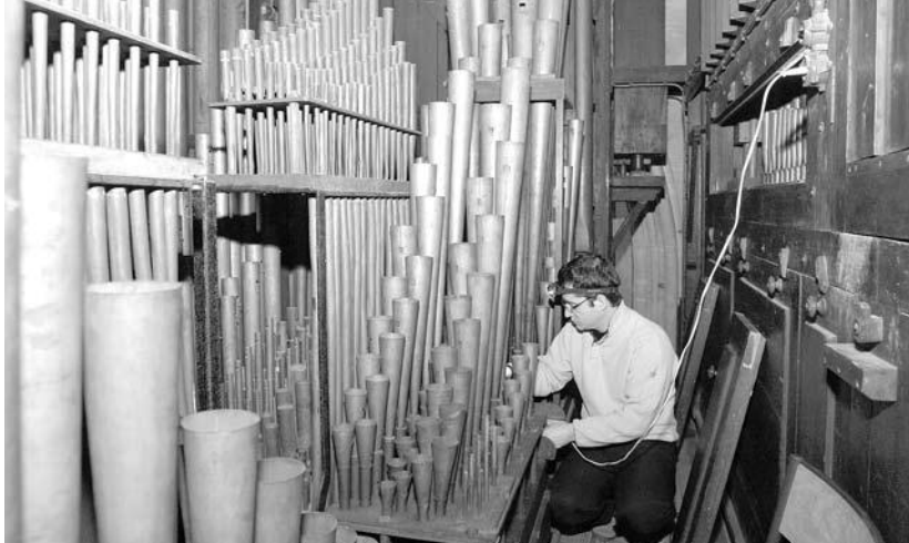
Denis Lacorre tuning the Bombarde Reeds at Saint-Ouen
